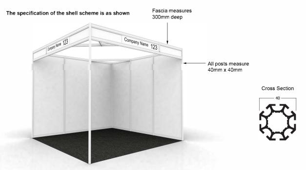
990mm centres between Posts 495mm centres between Posts Seen size 455mm x 2340mm Seen size - 950mm x 2340mm Cut size - 964mm x 2354mm Cut size 469mm x 2354mm 455mm between Posts 950mm between Posts 40mm x40mm Post
